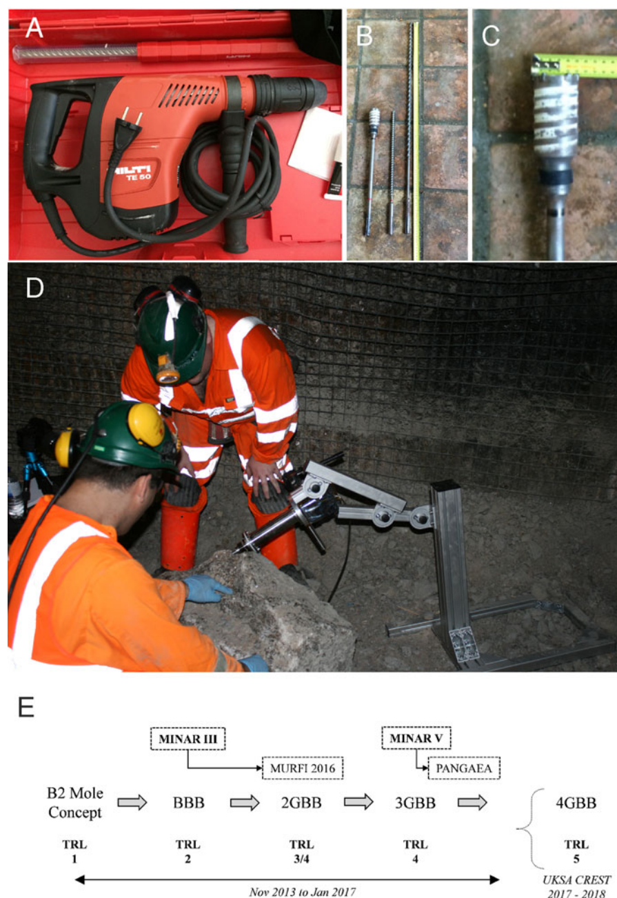
Fig. 4. Some of the sample acquisition instrumentation deployed in MINAR 5. (a)–(c) NASA drill. (a) The Hilti Drill TE 50, 1050 Watts; (b) 42 cm core string; 40.6 cm cutting string; 92.7 cm cuttings string; (c) core drill bit diameter 5 and 7 cm long, (d) The SPLIT instrument in operation on an artificial outcrop of halite in the Mars Yard; (e) the use of MINAR for the methodical development of the SPLIT technology (see ‘Results’ section for details).
